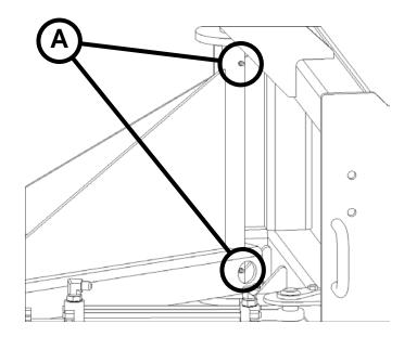
Use No. 2 lithium base gun grease when lubricating all the attachment grease fittings.
